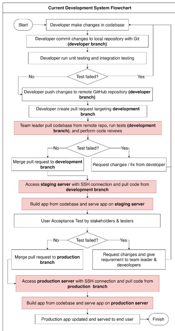
Figure 4. Current Development System Flowchart
