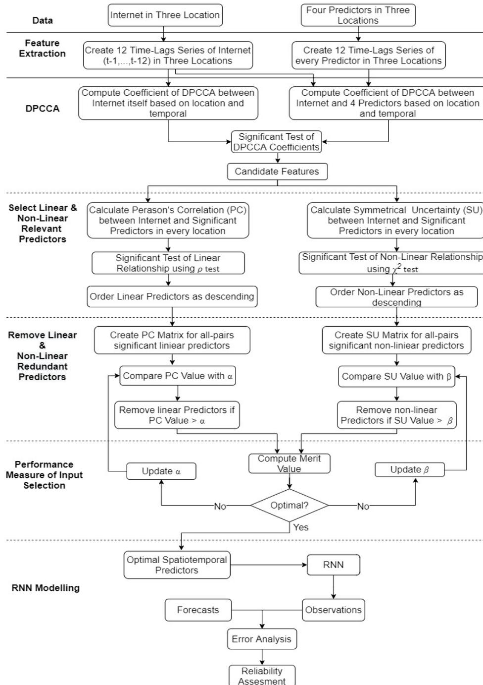
Figure 5. Complete flowchart proposed method
