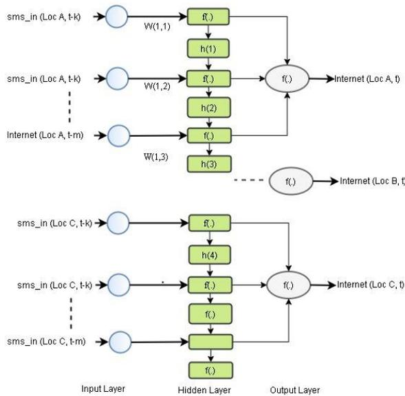
Figure 4. The architecture of RNN internet-traffic forecasting
