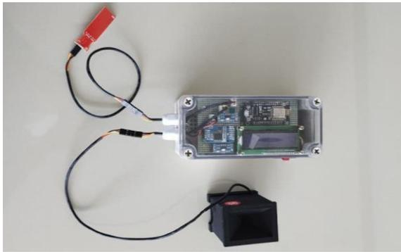
Figure 2. prototype of rainfall sensor
