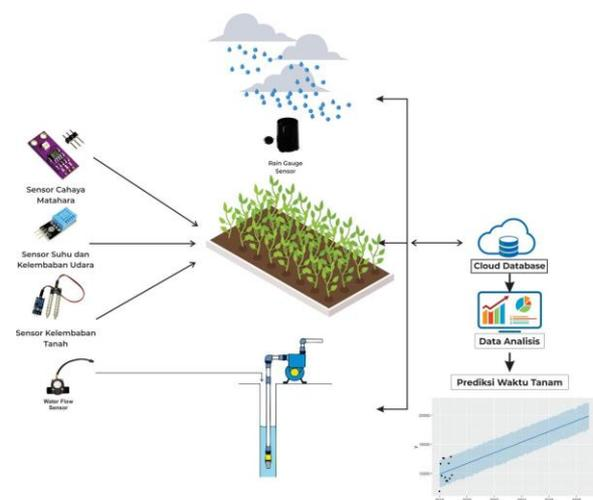
Figure 1. Design of the sensor that predicts the planting time of Tobasco pepper based on environmental conditions.
