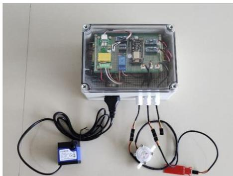
Figure 3. prototype of water flow sensor
