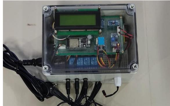
Figure 4. Prototypes of temperature sensor, air humidity sensor, and sun light sensor
