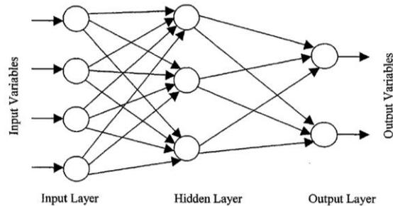
Figure 6. The Schematic representation of a three-layer neural network
