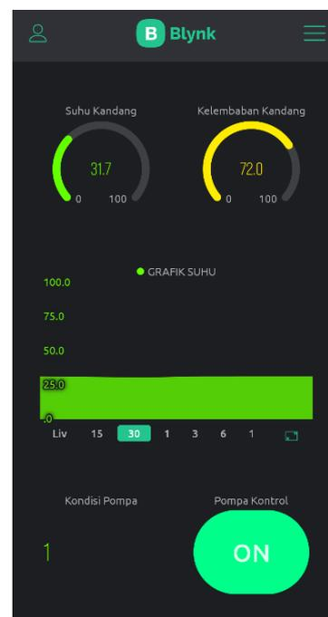
Figure 5. The display of monitoring and controlling the temperature and humidity of the cage when the DHT11 sensor detects a temperature over 30°C.
