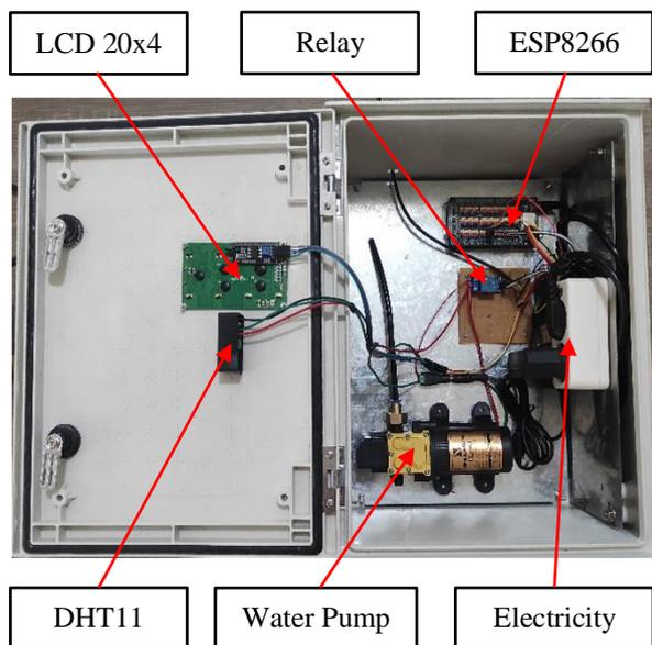
Figure 4. IoT control devices
