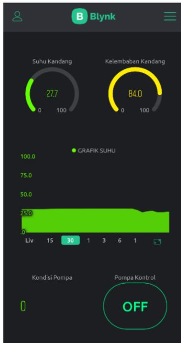
Figure 6. The display of monitoring and controlling the temperature and humidity of the cage when the DHT11 sensor detects a temperature less than 28°C.
