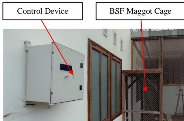
Figure 3. Maggot cage and IoT control device.
