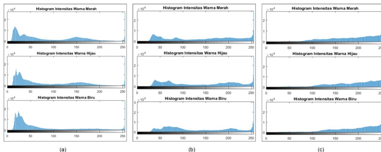
Figure 9. Distribution of RGB color intensity histograms (a) fresh, (b) started to rot, and (c) rotted
